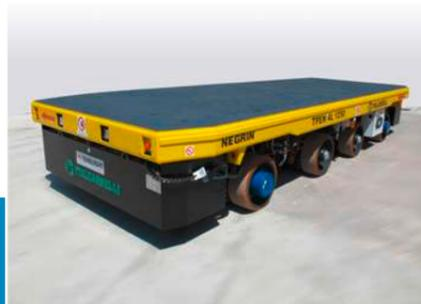
▣ *Italtcarrelli TPE 4L 1250 self-propelled platform transporter with 125t of load capacity remote controlled and with multidirectional steering system.*
