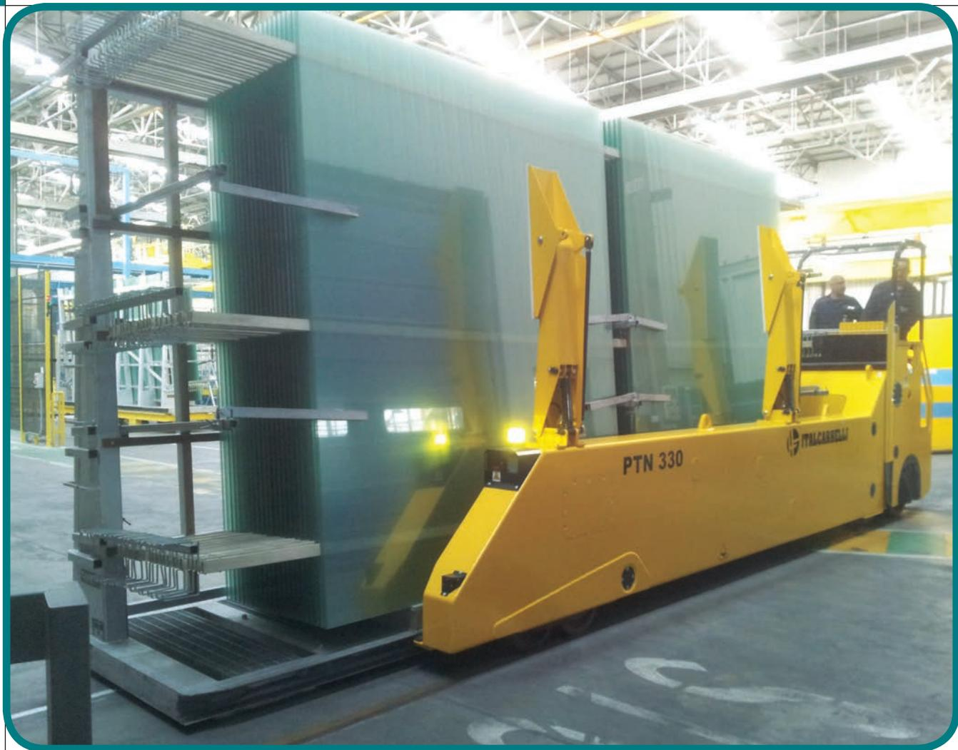
series of installations for automatic guiding, including a packaging line in a float line in Russia. This plant also includes one of our PTN330 inloaders, which have an optical guiding system that enables to automatically identify and follow a route painted on the floor. By means of this optical guiding system, the machine can also automatically and highly-precisely stop in an indicated position, ideal to place racks on automatic packaging lines, unloaders, transformation lines, etc.
